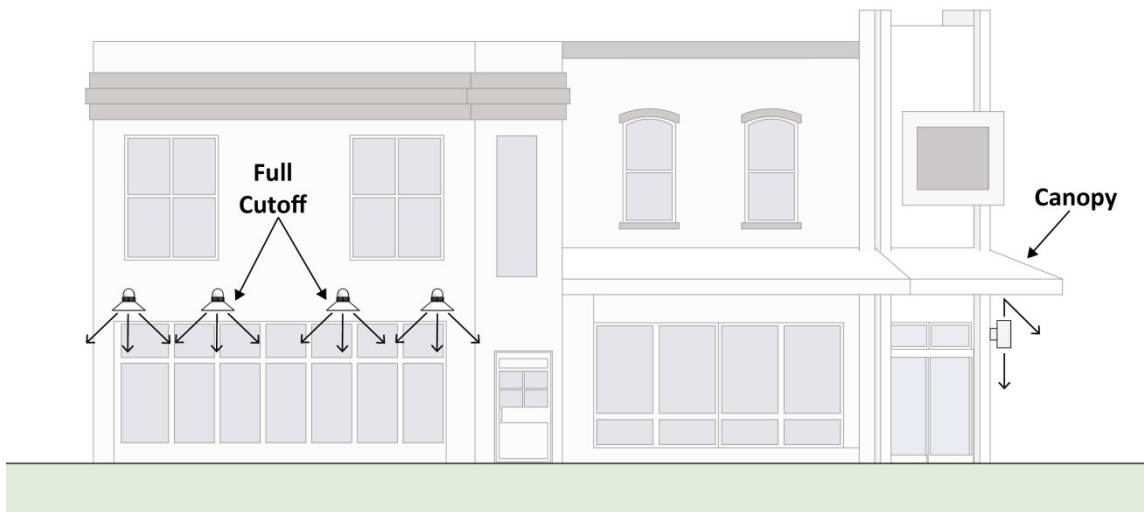
Figure 53: Exterior Light Shielding
